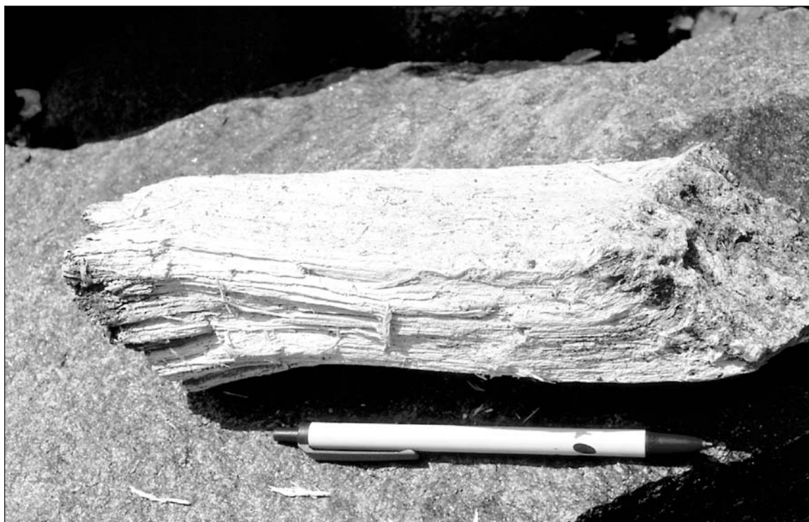
Figure 8. Photograph of a tremolite asbestos sample collected from a large vein within a serpentinite, Montgomery County, Maryland, USA. Pen for scale is 14 cm long.
