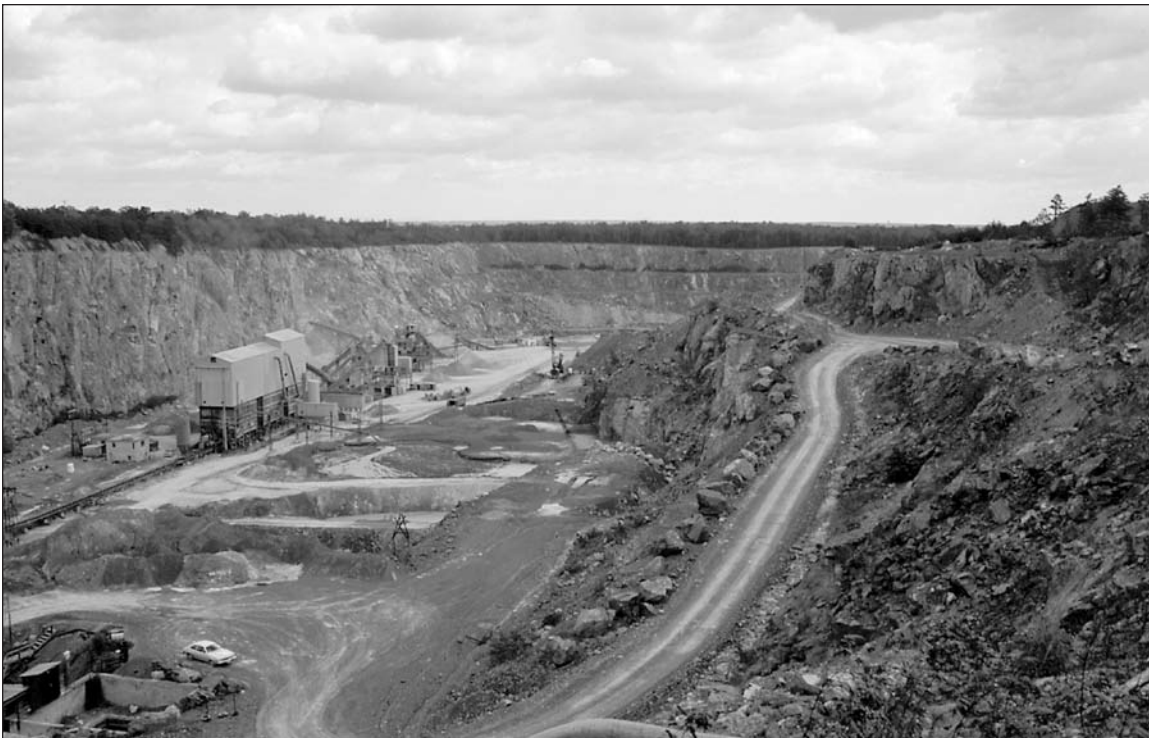
Figure 9. The Hunting Hill serpentinite quarry, near Rockville, Maryland, furnishes crushed stone to the Washington, D.C., metropolitan area. The quarry came into prominence in 1977 when chrysotile fibers were detected in dust emissions.
